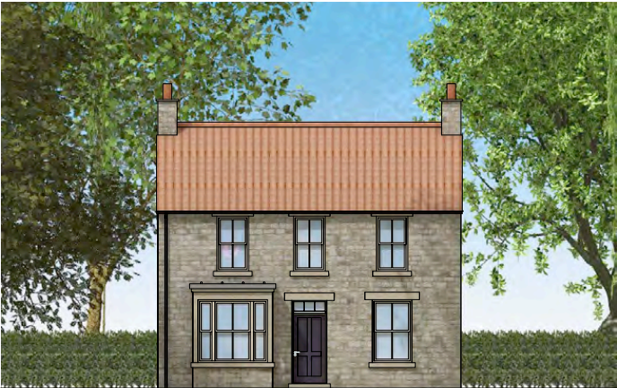
A | FRONT ELEVATION STUDY: HOUSE TYPE C 1:100 Natural stone & clay pantiles
