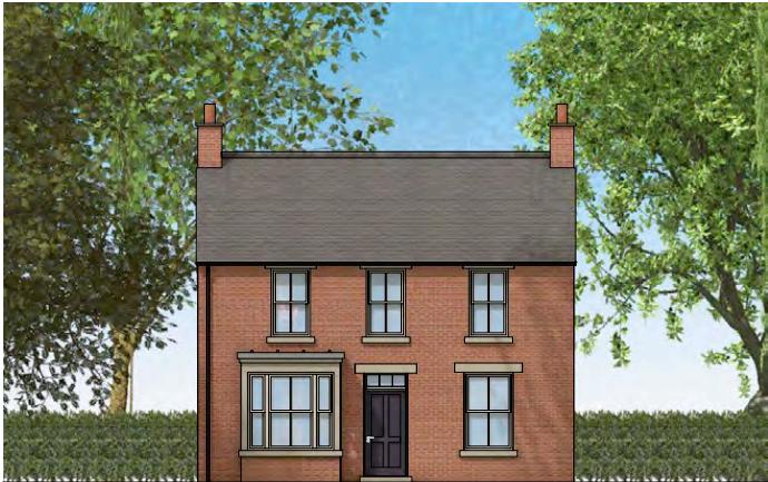
B | FRONT ELEVATION STUDY: HOUSE TYPE C 1:100 Clay facing brick & natural slate
